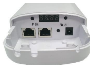
EZ-Bridge® 5AC Inside Connections
